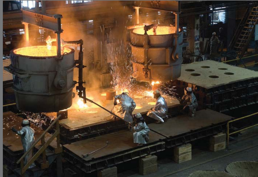
Shipbuilders pour rudder casting for the aircraft carrier Gerald Ford (CVN 78) at Newport News Shipbuilding.
