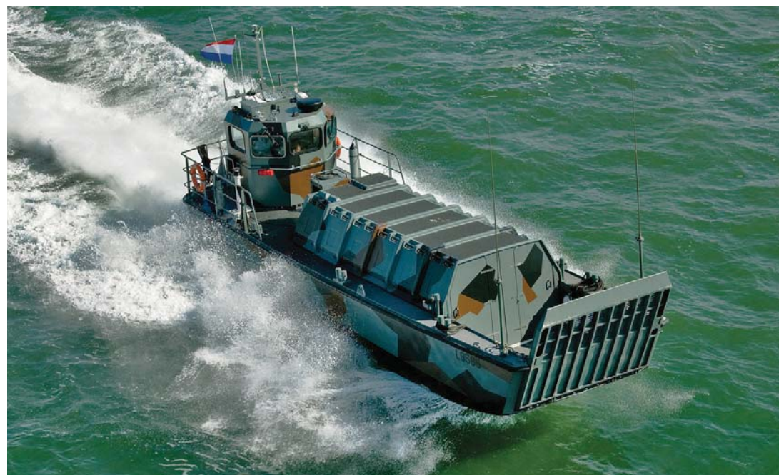
Dutch Navy Landing Craft is fitted with twin UltraJet 410 Waterjets.
