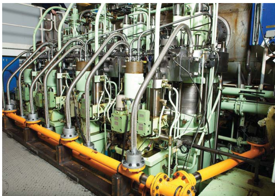
The new two-stroke ME-GI test engine has an integrated gas supply system.
