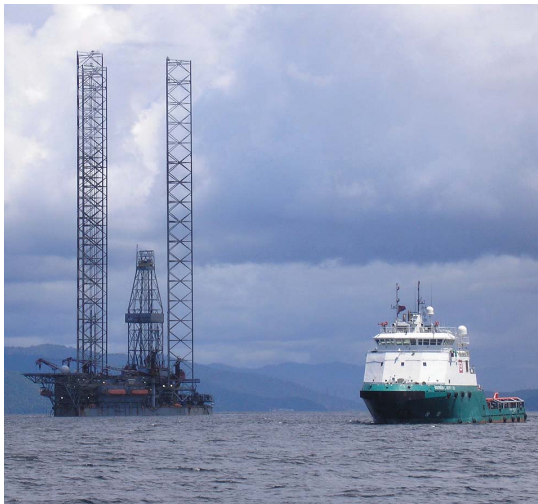
Platform towage operation with the AHTS Bourbon Liberty 205 at Trinidad and Tobago.
