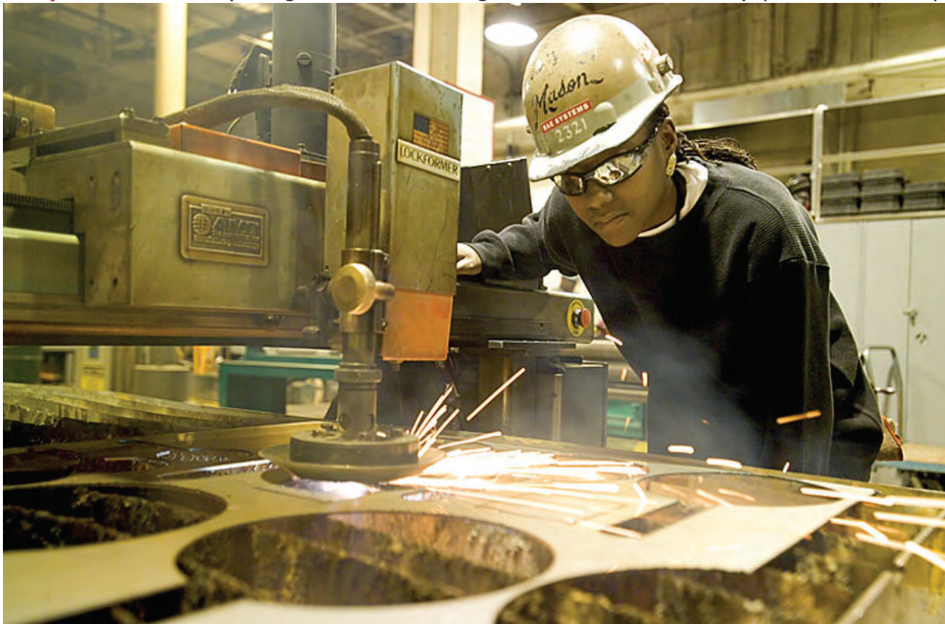
BAE Systems: Falon Mason operating the Vulcan CNC burning machine in the Sheet metal Shop. (Photo credit: Ed Ketz)
