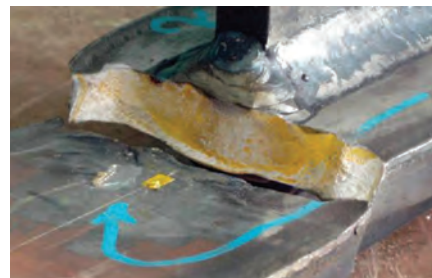
An example of steel fatigue failure after testing at low temperature
