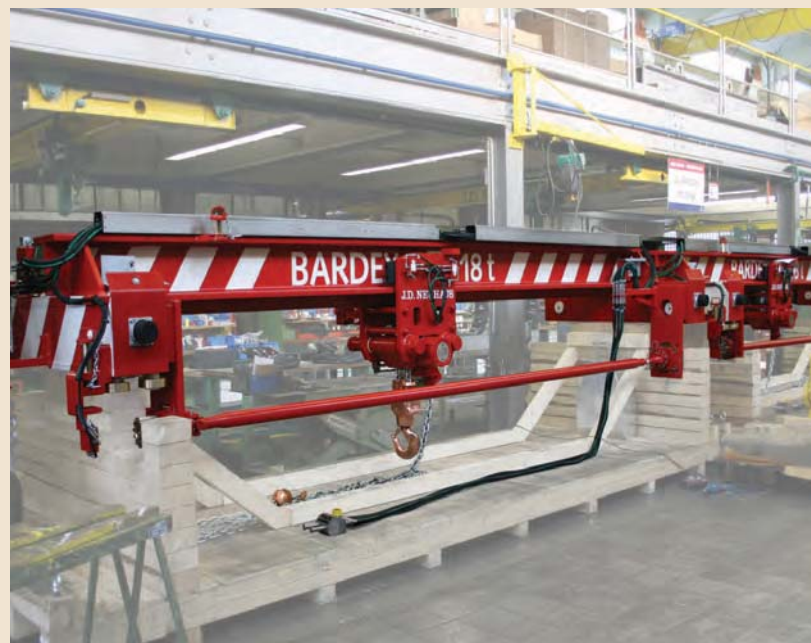
A hydraulically operated overhead crane with a hoist lift capacity of eight tons, manufactured by J D Neuhaus for Bardex Corp.
