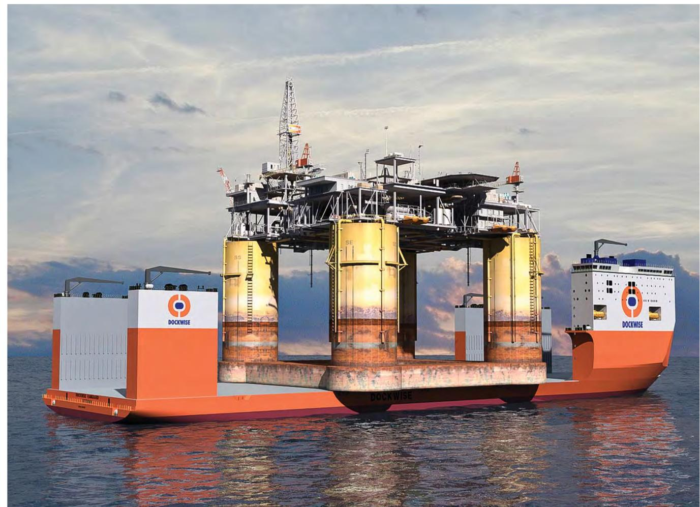
Dockside's new Super Vessel, Dockwise Vanguard presently under construction at HHI shipyard in Korea is due for completion in the latter part of 2012. It will have a capacity of more than 110,000 metric tons, and deck size of 900 x 230 ft (275 x 70 m).
