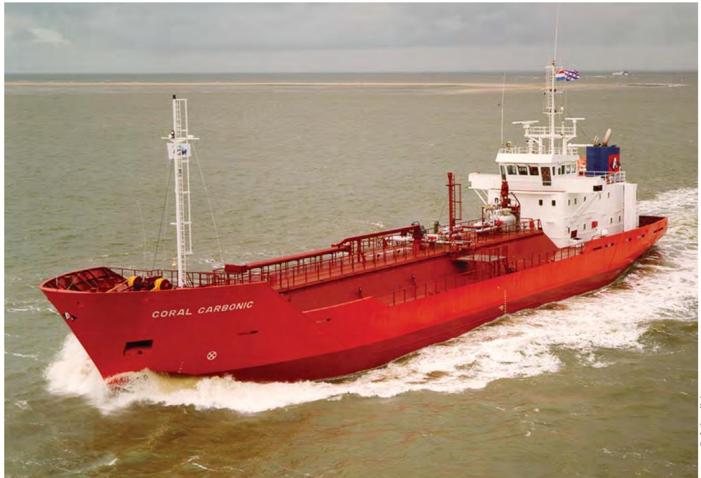
The 1,666-dwt, 262 ft. MV Coral Carbonic was built in 1999 for the transport of liquid CO2. The quality of the system ensures safe handling of the gas which can be used for human consumption and cannot be carried in other gas tankers.
