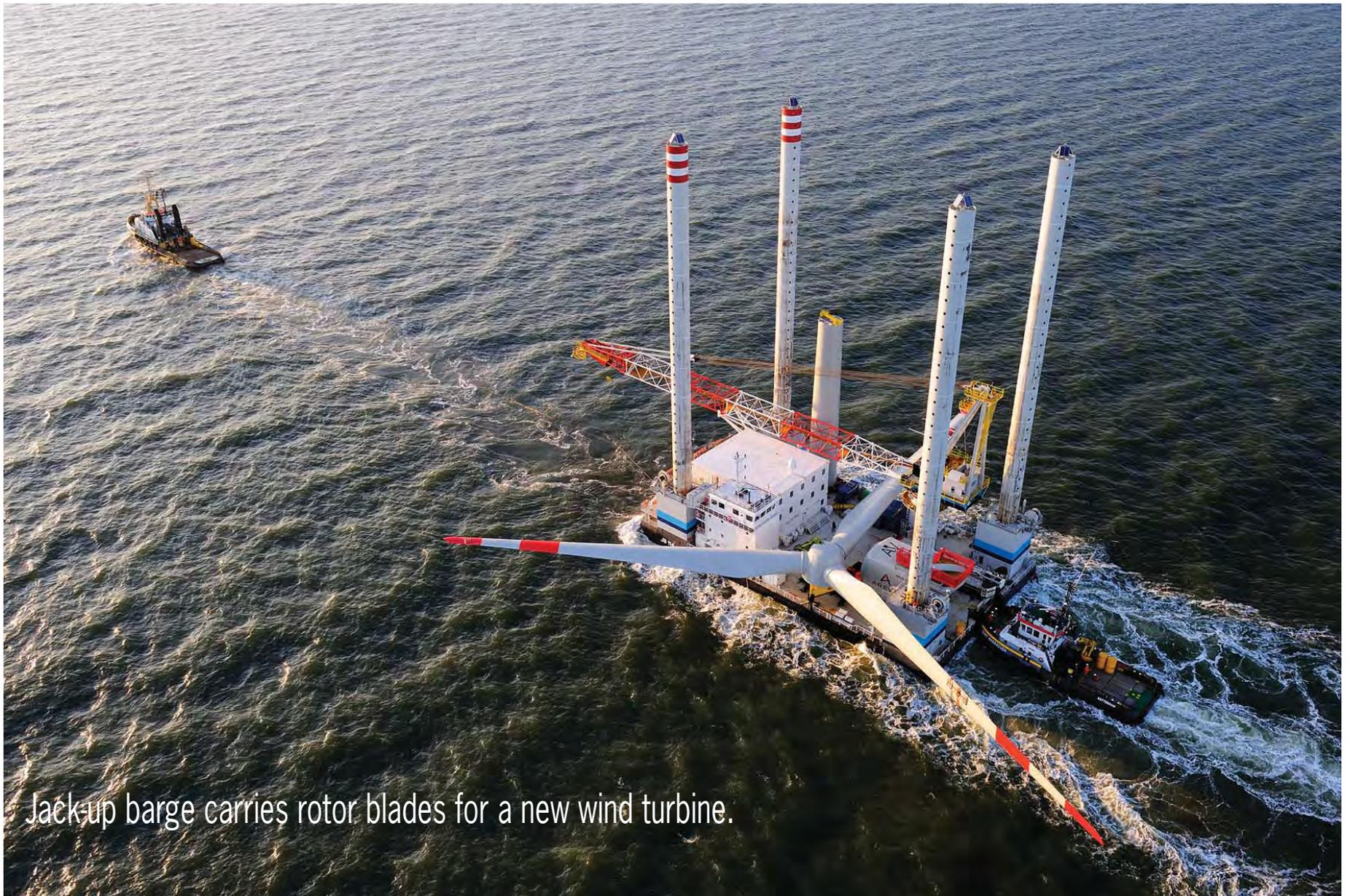
Jack-up barge carries rotor blades for a new wind turbine.
