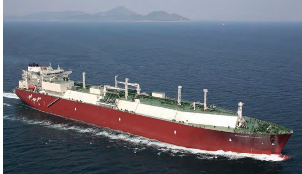
Built by DSME the Woodside Rogers LNG carrier is equipped with a GE electrical induction-based propulsion solution.
