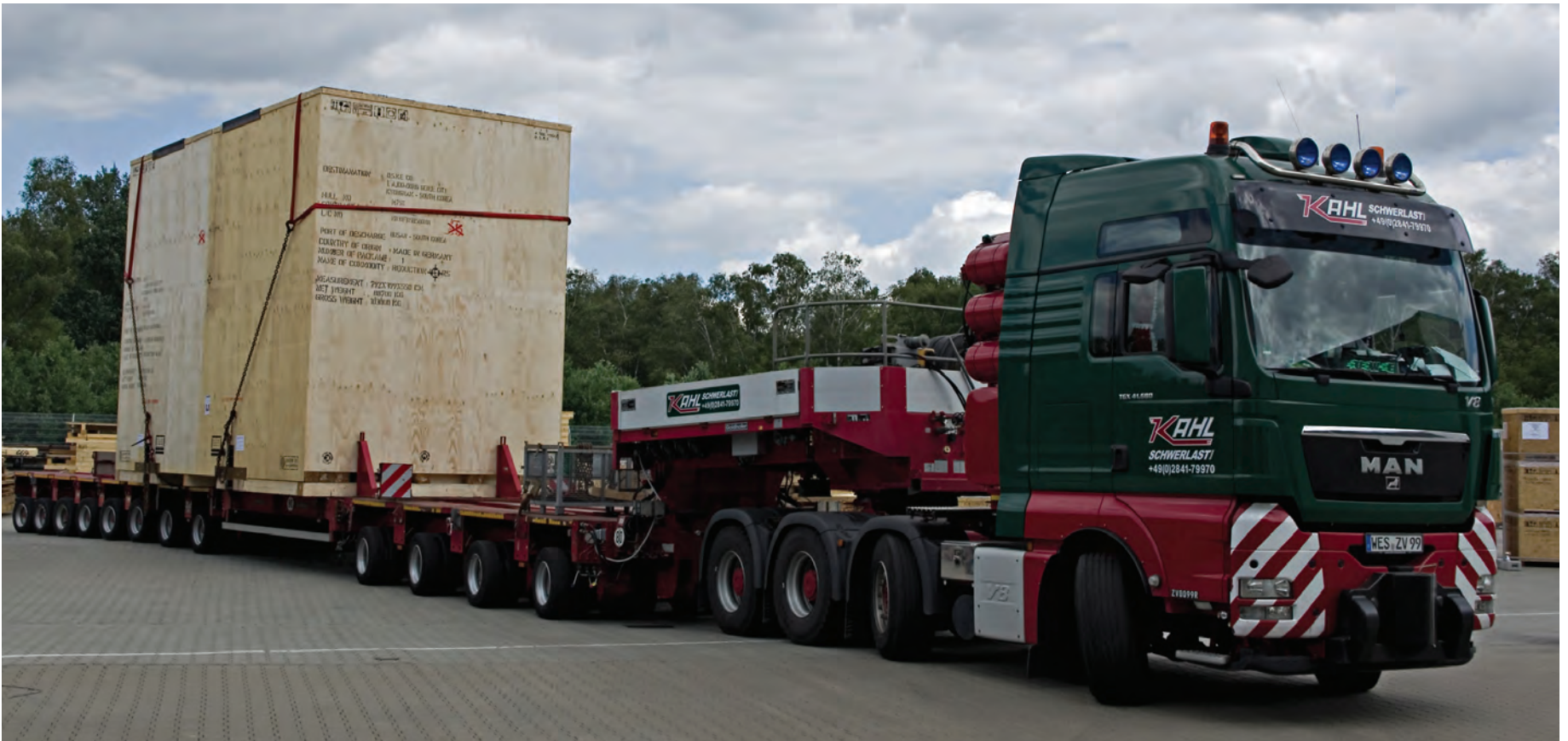
Fig. 5: With dimensions of 7.35 x 4.92 x 3.7 m and a weight of 89 tons the transport of the two type Navilus GVLQ 2500 multi-engine gearboxes alone is a masterly piece of logistics. (Source: Siemens)
