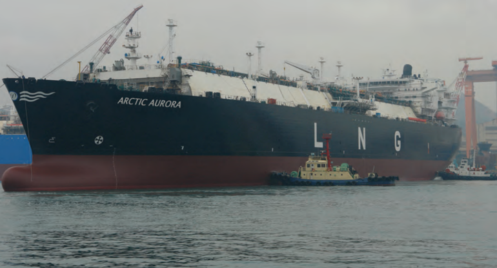
Arctic Aurora, the second of two new ice-class LNG carriers for Dynagas built by Hyundai Heavy Industries.
