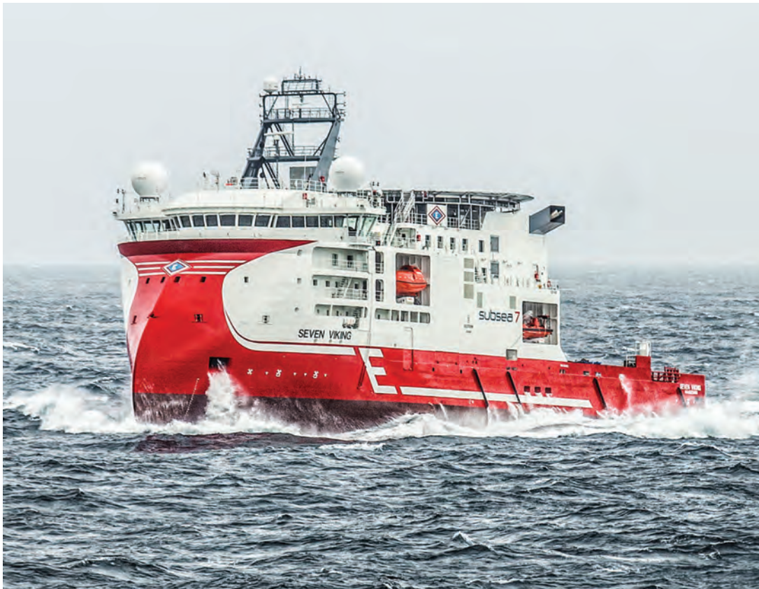
Incorporating the X-Bow design, the inspection, maintenance and repair vessel Seven Viking was built for Subsea 7 and Eidesvik and entered service in 2013.
