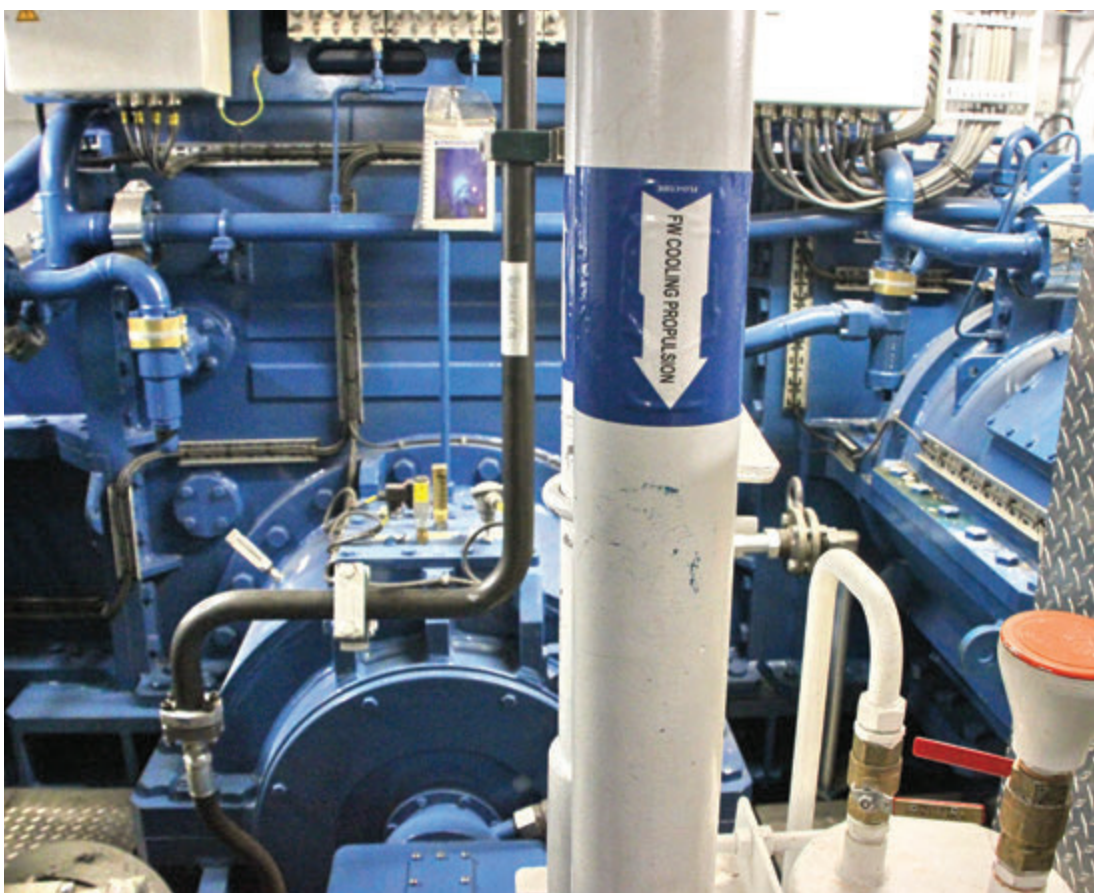
Below: The Renk MAN gearbox combines the power of two gas engines.
