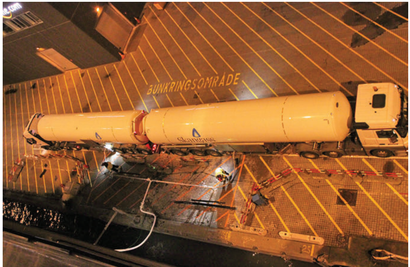
LNG-bunker procedure by trucks during embarkation of passengers in Hirtshals.
