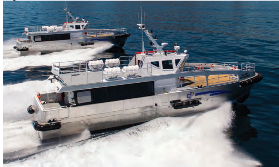
Sign of the Times ... Bulletproof pilothouse on 20m Crewboats
