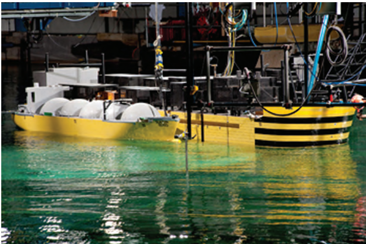
A scale model of the FLNG measures 8 meters long and weighs 4.5 tons.
