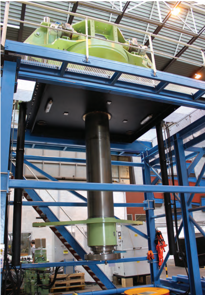
The 2MW Retractable Azimuth Thruster – the largest retractable unit in the ZF Marine Krimpen repertoire – for installation on a new U.K. military tanker.
