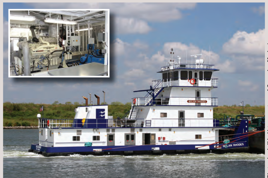
The Nolan Rhodes, from the John Bludworth yard, on the job for Enterprise Marine Services near Channelview Texas. Inset: Cummins engine and Z-drive on the Terry H.
