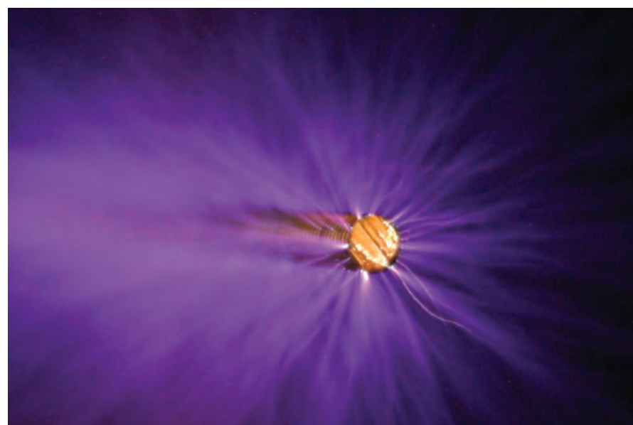
Long exposure photo of transient plasma streamers generated by multiple shots with a large air gap.
