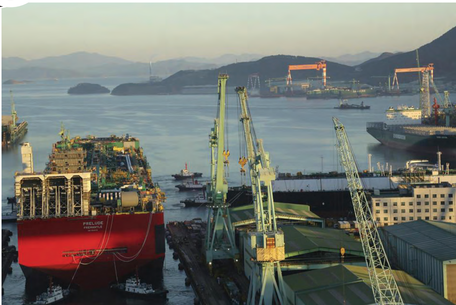
The 488-m hull of Shell's Prelude FLNG plant floating out of the dry dock at Samsung Heavy Industries.
