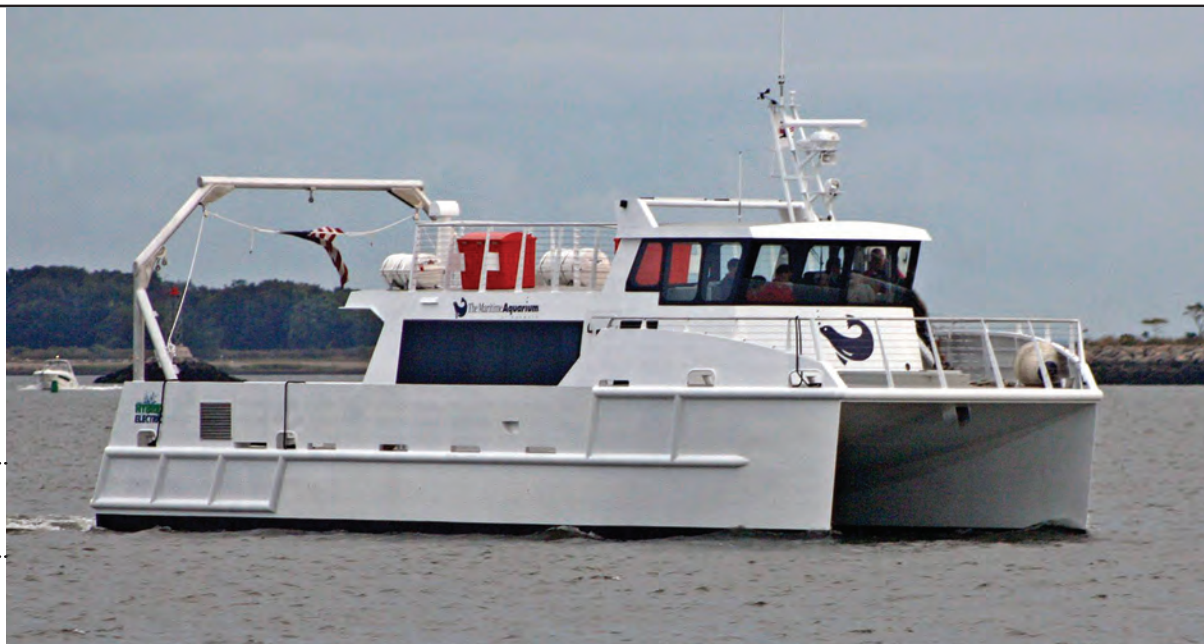
The 19 m research vessel ‘Spirit of the Sound’ runs virtually silently on hybrid electric power for two-hour study cruises on Long Island Sound.
