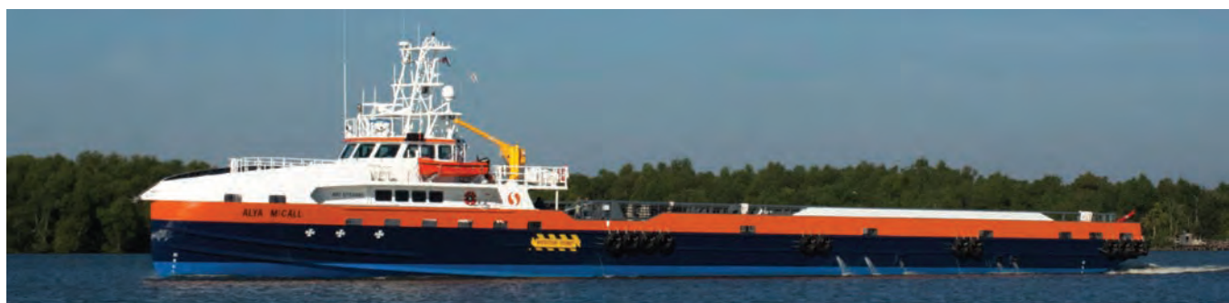
M/V Alya McCall | 206', 100 Passenger, DP-2 Monohull Fast Support Vessel Builder: Gulf Craft LLC Operator: SEACOR Marine Speed @ 50t deadweight: 38 knots
