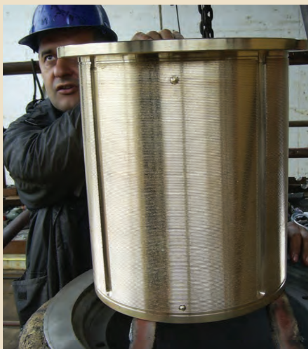
Picture 3: Bronze bearing machined and ready to be inserted in to the housing.
