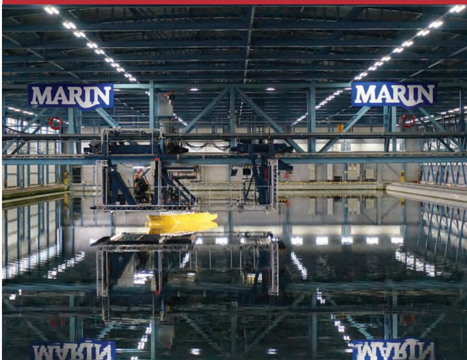
Example of a ship being tested with the use of MARIN's computerized planar motion carriage. This methodology works for model sizes between 2 and 10 meters.
