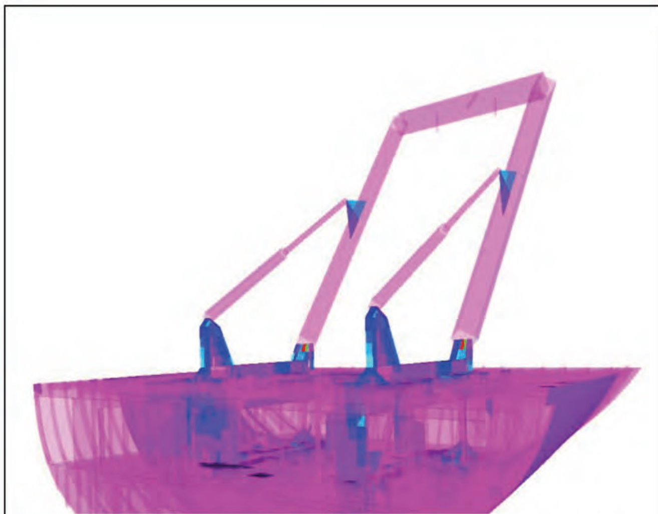
Figure 1 – A-Frame Initial FEA Stress Results
