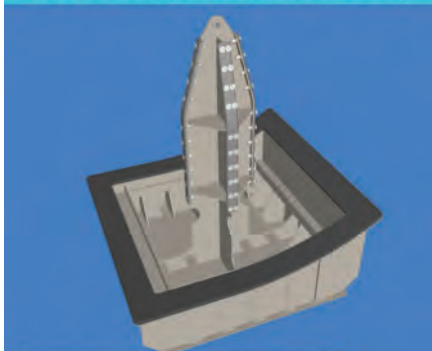
Cofferdam designed using scan data
