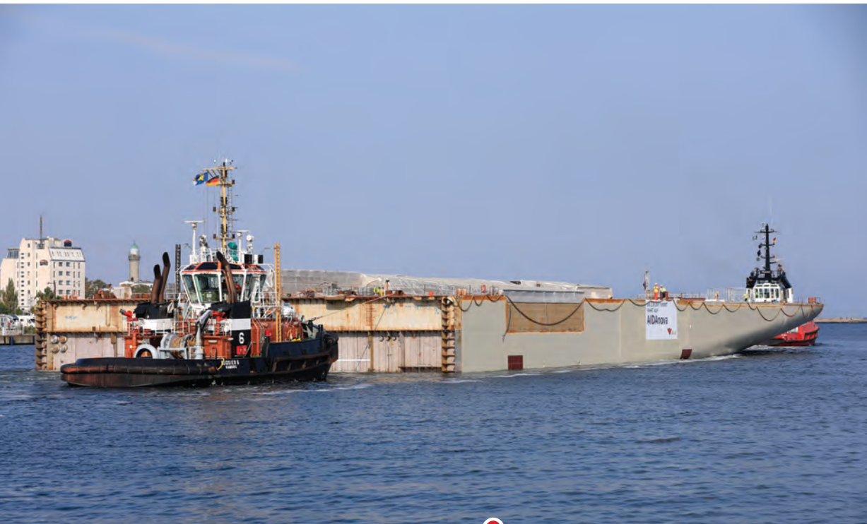
The first Floating Engine Room Unit (FERU) on its way from Rostock to Meyer Werft Papenburg.
