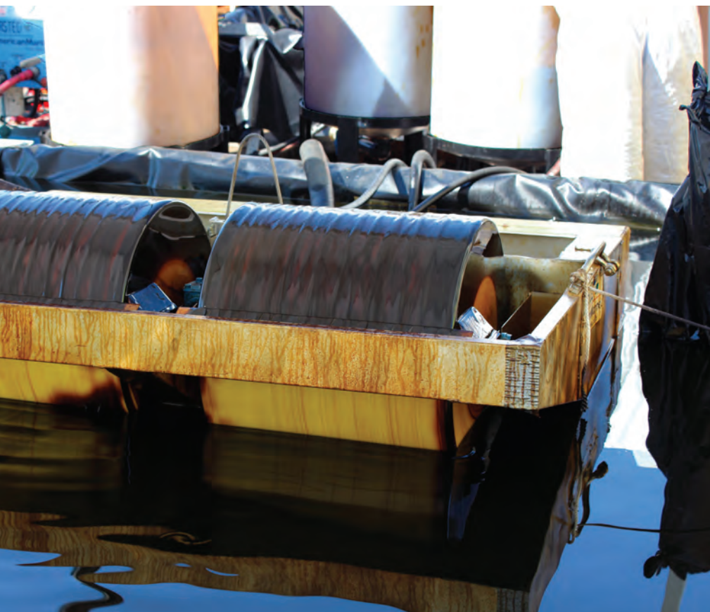
A skimmer was tested in controlled conditions to evaluate the impact dispersant mixed with crude oil has on skimmer performance.
