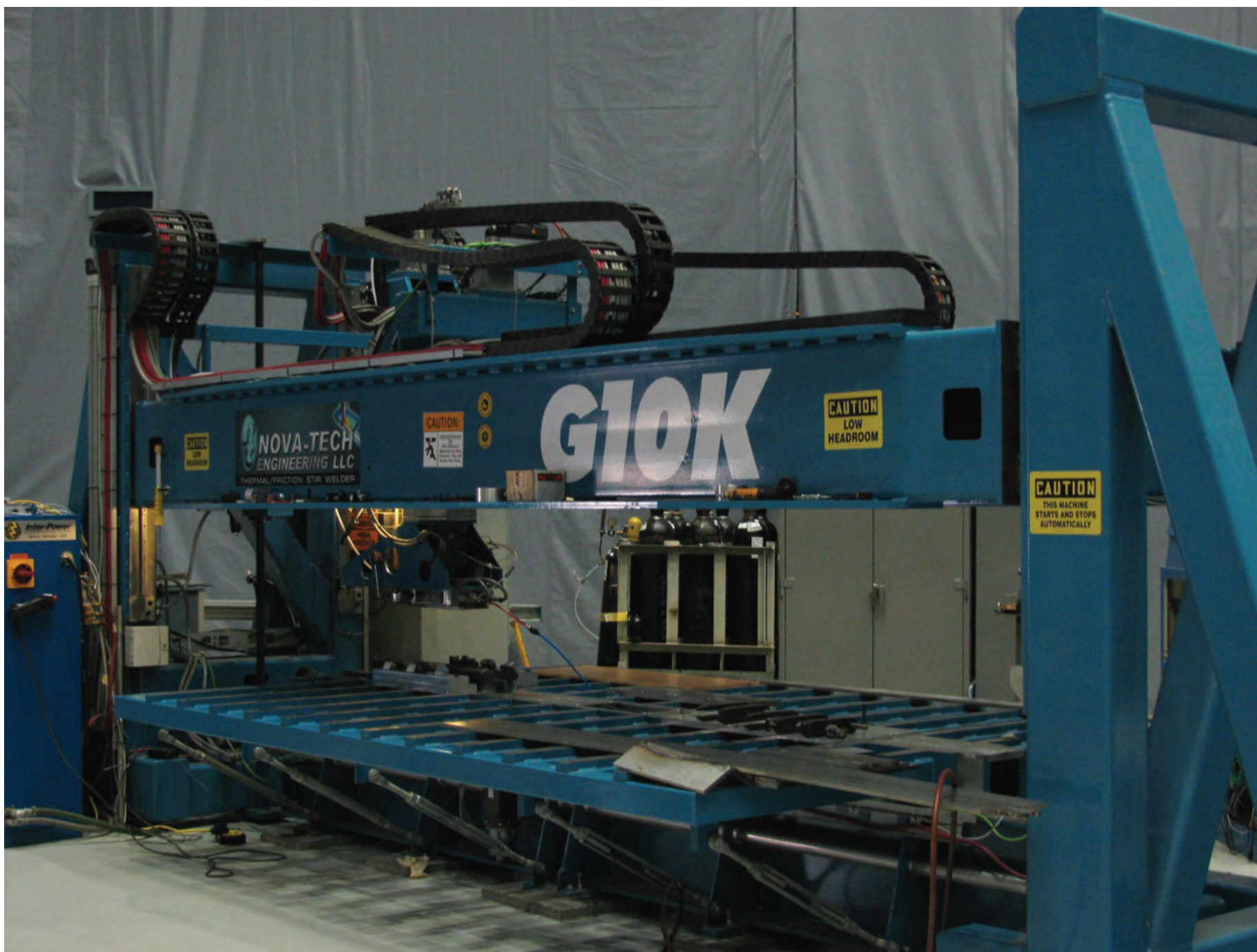
Figure 2 TSW Gantry Machine Used for Titanium Welding at MSFC
