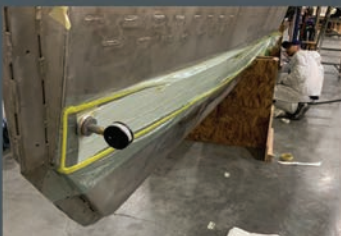
Welds being tested for the U.S. Coast Guard
