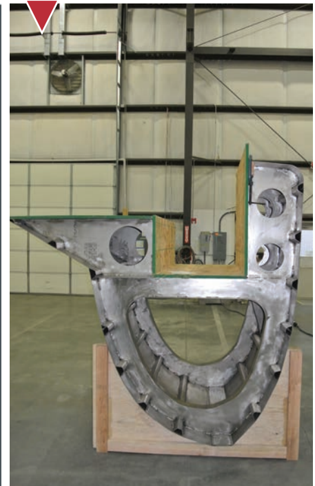
50 ft Titanium Sailing Catamaran Demi-hull Mock up Note Trapezoidal shaped stringers at Bettsboats Anacortes WA
