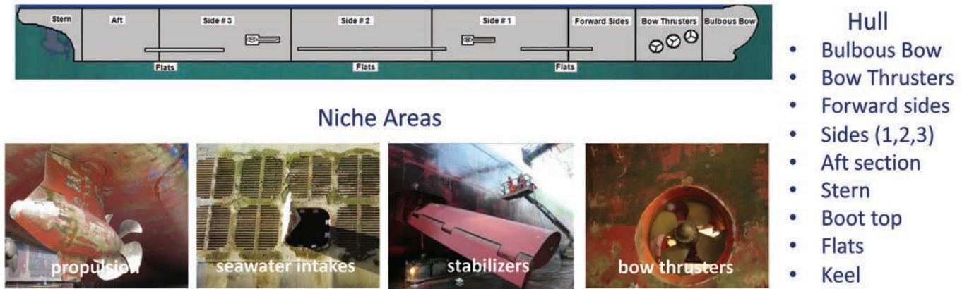
Figure 5. The general hull and niche areas of a ship.
