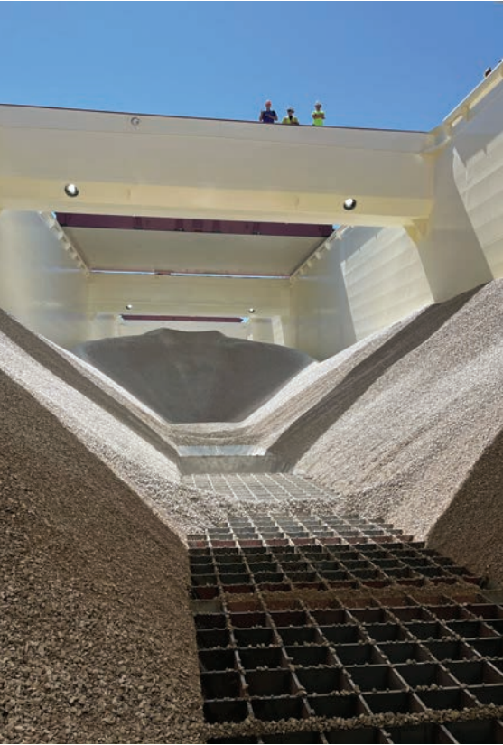
Figure 2. Distinguished by its square-shaped cargo holds, the vessel can transport a greater freight load than some larger vessels.
