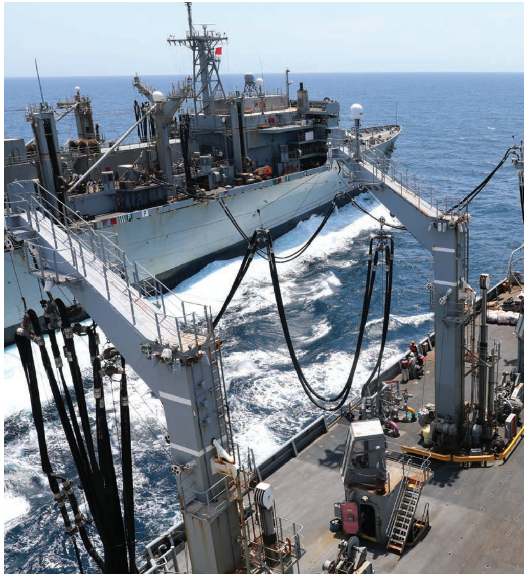
Military Sealift Command's fleet replenishment oiler USNS Joshua Humphreys (T-AO 188) sends fuel to MSC's fast combat support ship USNS Arctic (T-AOE 8) during an underway replenishment at sea in the Atlantic Ocean, July 17.
