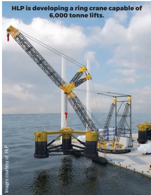
HLP is developing a crane that will enable components such as towers to be stacked vertically in marshalling areas.
