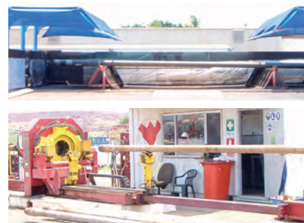
Figure 2. Weatherford used the operator's operations base to prepare and make-up tubular doubles prior to deployment.
