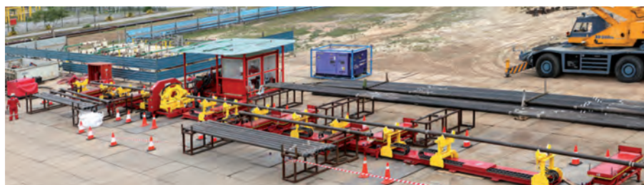
Figure 1. A Weatherford ComCAM onshore bucking system can make-up 5.5in diameter drillpipes in double or triple joints per stand, delivering substantial savings to operators in their transportation and downhole deployment costs.
