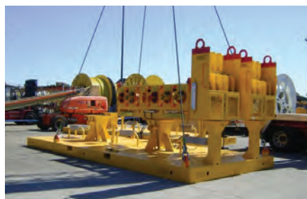
Umbilical distribution manifold at LLOG’s Who Dat development is tied back to its own floating production system, the only privately owned floating production system in the world.
