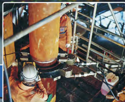
A Tri Tool® 600 Series Split-Frame Lathe performing a precision in-place sever on an offshore platform.
