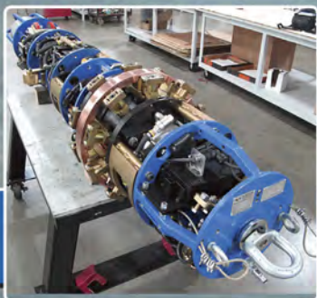
The powerful Tri Tool® ILUC 1820 configured for offshore pipelay project deployment.
