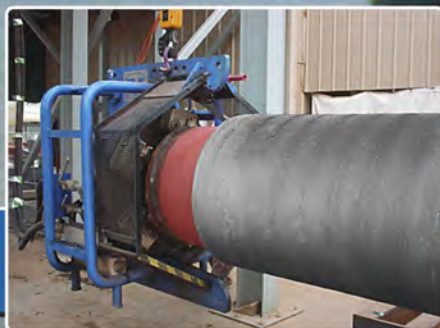
The rapid, reliable 16" to 32" PFM 1632 PIPEMASTER® facing concrete coated, large diameter flowline piping.
