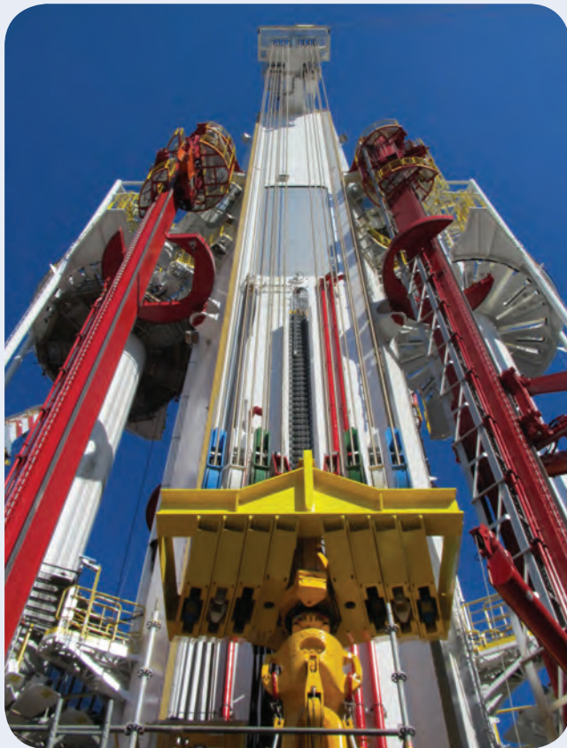
Looking up at the dual hoists flanking the multi-purpose drilling tower on the Noble Globetrotter .
