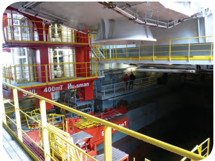
The Noble Globetrotter II has a large moonpool, over which the BOP is skidded and lowered.
