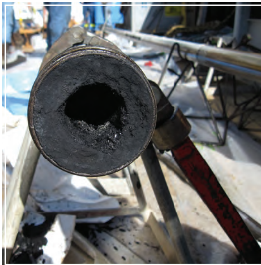
Bailer section packed with dense asphaltenes after the filter is removed. Asphaltenes set once exposed to lower temperature; when in the well under a certain temperature the asphaltenes are stickier.
