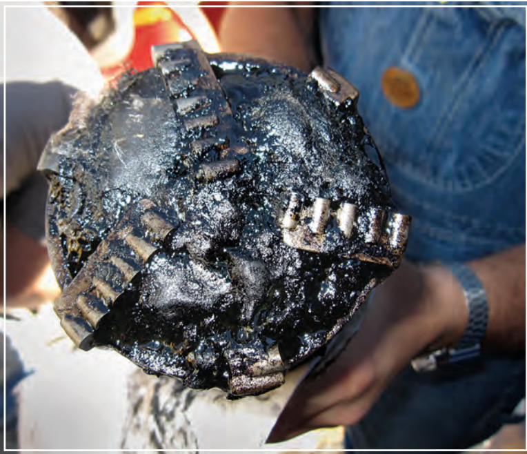
Milling bit packed with set asphaltenes.
