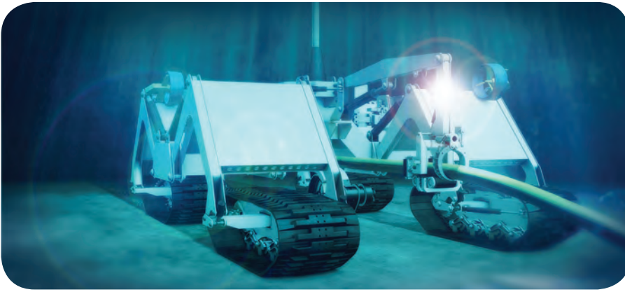
IHC Engineering Business' designed the Hi-Traq inter-array cable trenching machine.
