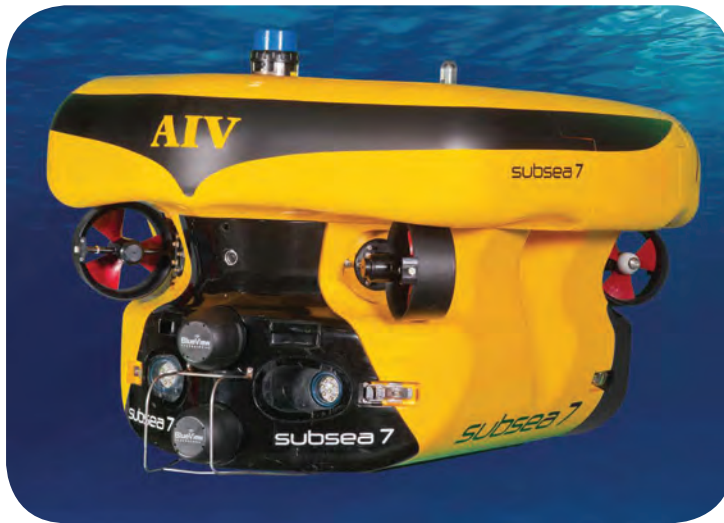
Subsea 7's autonomous inspection vehicle (AIV) designed in collaboration with SeeByte. Photo: Subsea 7.
