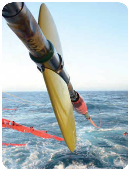
The multisenor streamer system deployed offshore Canada to acquire an IsoMetrix marine isometric seismic survey. Photo: WesternGeco.
