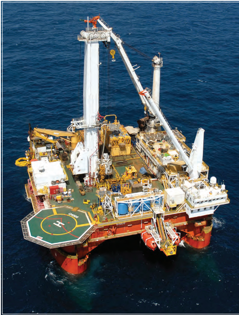
Open decks and sizable cranes aboard the vessel provide more efficient mobilization. Photo: Helix ESG
