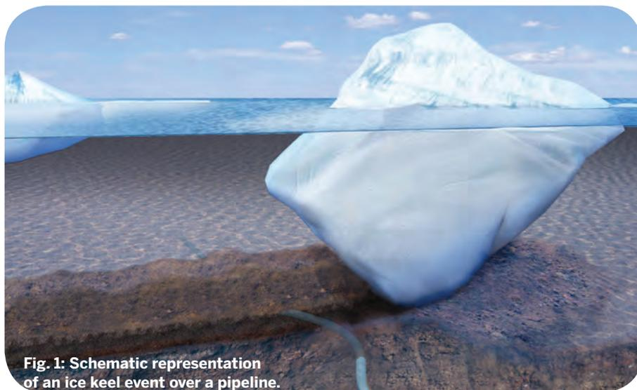
**Fig. 1: Schematic representation of an ice keel event over a pipeline.**
