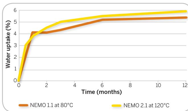
**Fig. 5: Water uptake in NEMO 1.1 and 2.1 during hot-wet exposure at 80°C and 120°C, respectively.**
