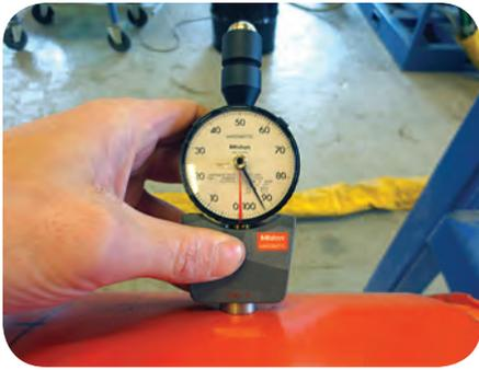
**Fig. 6:** Shore A Hardness Durometer is used to measure the hardness of the joint after demold time and after 24hr. The acceptance criterion is  $\geq 55$  at demold and  $90 \pm 10$  Shore A after 24hr.
