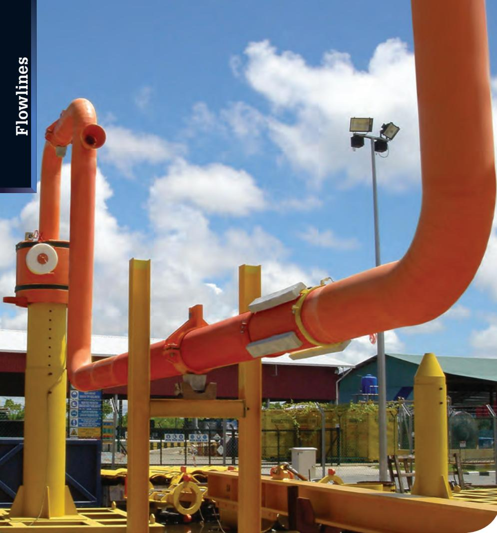
**Advanced epoxy coating can be used for coating all subsea equipment, including jumpers.** All images: Bredero Shaw
