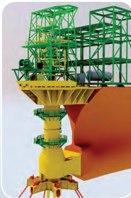
**A schematic of LMC's external turret system design for the FSRU *Toscana*.**
