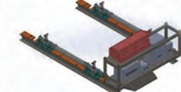
Skidding system with locking mechanism and wireless handheld controls on vessels.
