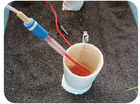
**Fig. 8:** A 100mm x 100mm test specimen of NEMO 1.1 was setup for a cathodic disbondment test for 28 days at 95°C in 3% NaCl solution and -1.5V. The average disbondment was 8.8mm and met the acceptance criteria of  $\leq 20$ mm.
