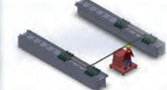
Skidding system with locking mechanism on vessels.
