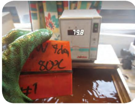
**Fig. 7:** A 100mm x 100mm test specimen of NEMO 1.1 was immersed in the water bath at 80°C for 48hr. There was no edge disbondment and passed the acceptance criteria with Rating 1.
