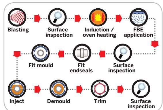
**Fig. 3:** The NEMO system coating application process.
