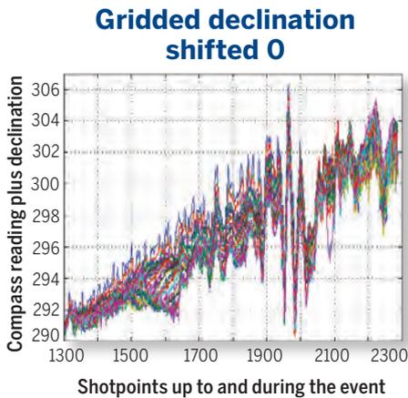
**Fig. 6: Compass readings corrected with gridded declination versus shotpoints**
