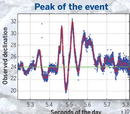
improvement of real-time declinations over modeled declinations for marine seismic streamer positioning in the Arctic.
