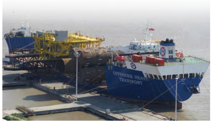
**FIG. 4 & 5: TRANSPORT ARRANGEMENT AND SKID-OVER MATING WITH TOPSIDE SUPPORT FRAME**
