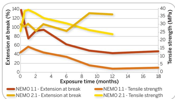
**Fig. 4: Aging tests for NEMO 1.1 at 95°C and NEMO 2.1 at 120°C.**
