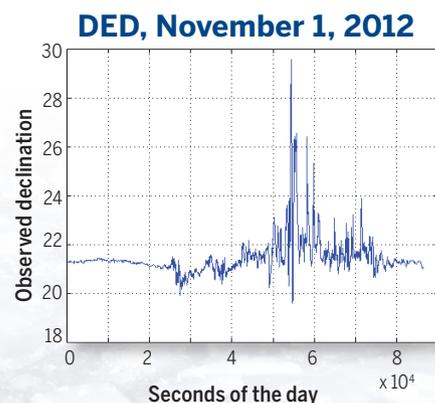
**Fig. 4: Declination (adjusted for baseline) measured at DED on the day of the event analyzed.** Source: ION.
