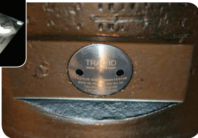
A stainless steel identification plate, and a drill pipe tag fitted with RFID.
