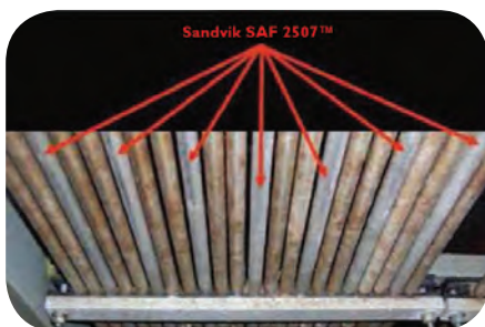
Fig. 2: ASTM 316L stainless steel and SAF 2507 super-duplex tubing, installed side by side, with the ASTM 316 tubing showing extensive corrosion and the super-duplex tubing showing none.
