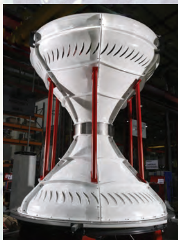
Dresser-Rand's HydroAir turbine design that can be incorporated into an OWC structure.
