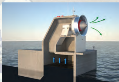
As waves pass, the water column moves up and down. Air is compressed and is driven through the turbine under pressure, generating electricity (pictured left). As waves recede, air is sucked back into the OWC, continuing the electricity generation (pictured right).
