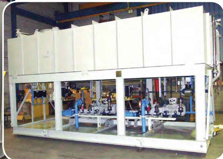
Litre Meter VVF meters on a Geveke Pompen chemical injection skid.
