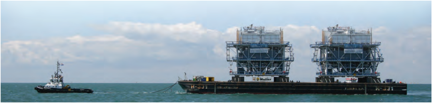
The two London Array wind farm substations, pre-wired, en-route for offshore installation. Photo courtesy of London Array Limited.
