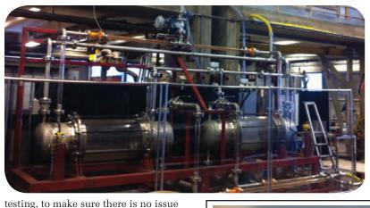
The gas pressure pump during proof of concept testing. Photos from Aker Solutions.
