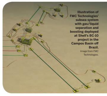
first such system to boost production of a mature field that also includes the reinjection of previously-removed water.
