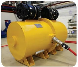
A scaled-down Rotoconverter prototype.
