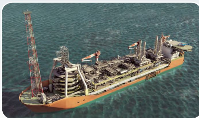
BP’s Quad 204 redevelopment will use a new FPSO and polymer injection is being investigated for EOR. Photo from BP.
