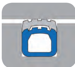
Figure 2: High-pressure seal profile
