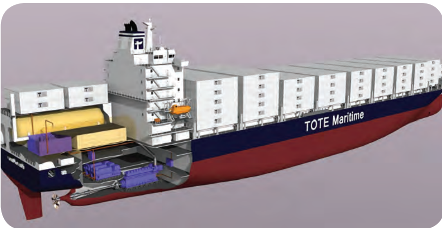
JMU says the shape flexibility of the IHI-SPB makes it an ideal alternative to the Type C tank, shown here in concept renderings for TOTE's gas-fueled containerships and Waller Marine's articulated tug barges. Images courtesy of TOTE and Waller Marine
