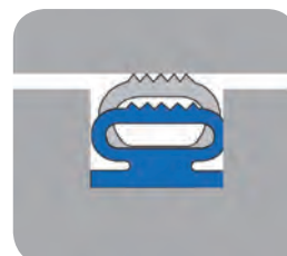
Figure 3: Low-pressure seal profile
