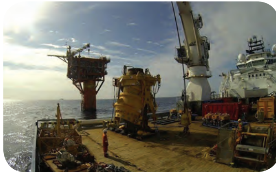
The clamp on deck, with the Varg A monotower in the background. Photos from IK.
