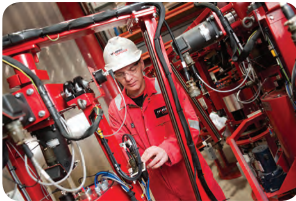
A Harris CapRock technician prepares a stabilized antenna system for advanced VSAT deployment. Photo from Harris CapRock.
