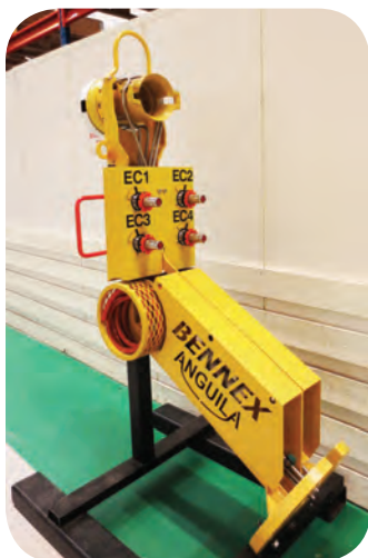
Bennex Anguila cobra heads can contain up to 13 precision-bent hydraulic tubes. Photos from Unison.
