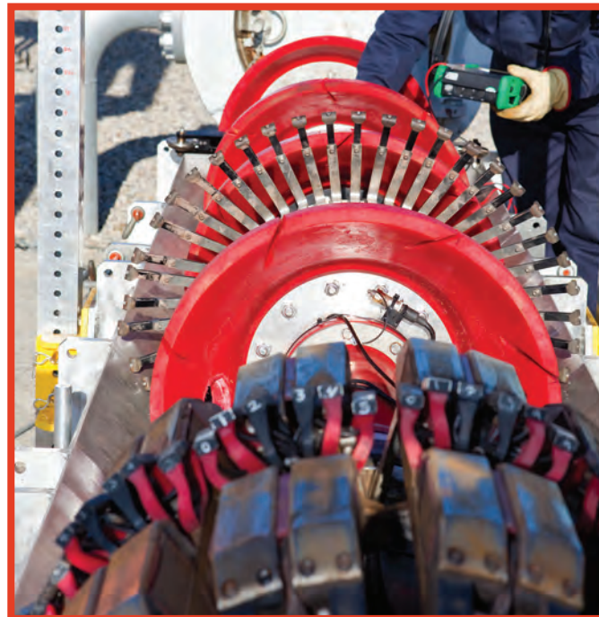
Intelligent PIGS can be used to assess internal corrosion.
