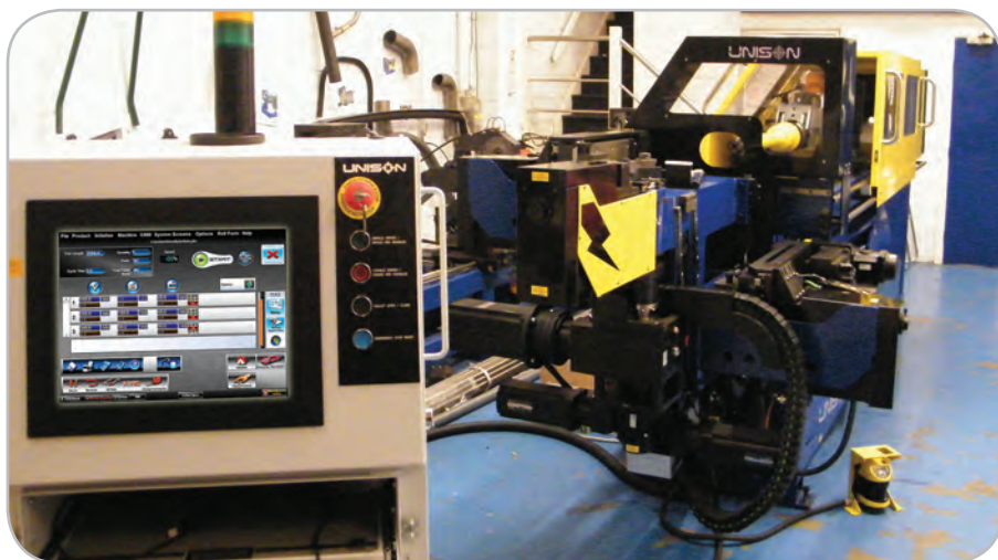
The tube bending machine undergoing final commissioning checks at Unison's UK manufacturing facility, prior to shipment.
