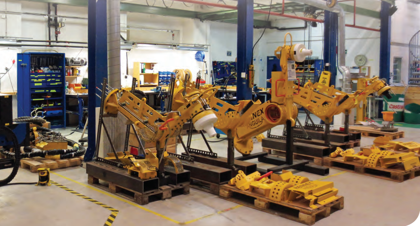
Siemens Subsea Products' hydraulic workshop in Norway uses this Unison tube bender for all small-bore tube fabrication.
