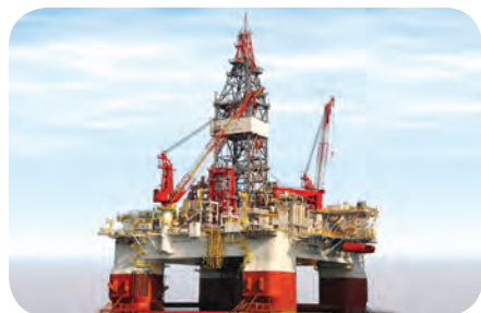
Transocean's West Capricorn drillship is capable of operating at 10,000ft water depth and drilling down to 37,500ft.
