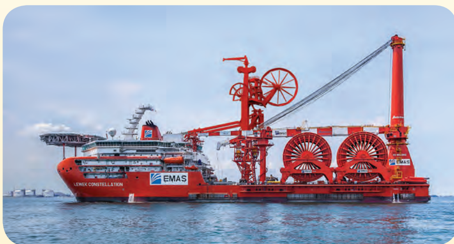
EMAS AMC's newbuild Lewek Constellation , which is having its multi-lay tower installed at Huisman's yard, Rotterdam, in November. Image from EMAS.
