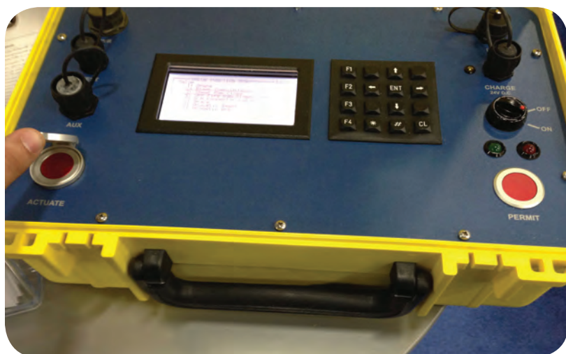
A topside acoustic system used to engage subsea accumulators.
