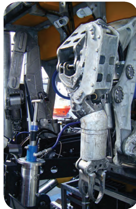
17H hot stab mounted on an ROV's porch. Photo from Reaching Ultra.
