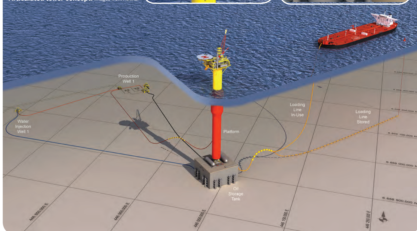
Articulated tower concept. Images from Atkins.
