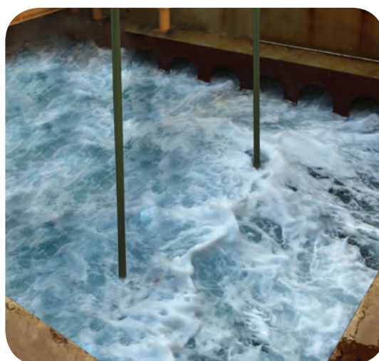
Coiled tubing running through a vessel's moonpool.
