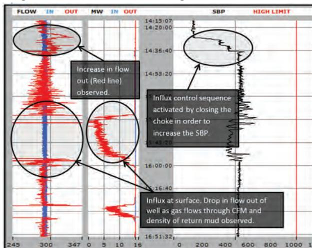
**MPD screenshot demonstrates flow into the well and increase in flow out of the wellbore, with the SBP required to control the influx visible in the third column.**
