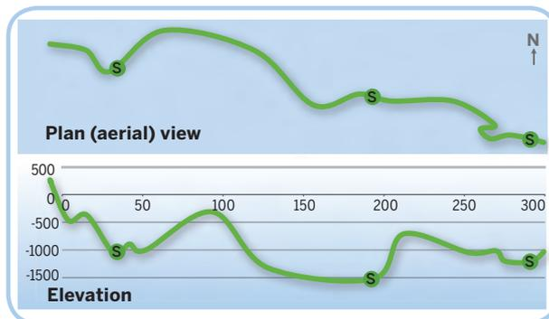
Possible pipeline route with tie-in points for subsea pressure boosting.
