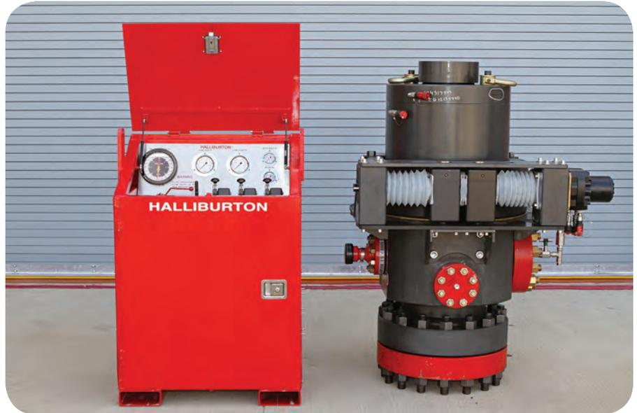
**RCD5000 Big Bore with the hydraulic clamping device standing beside a hydraulic closing unit.** Photo from Halliburton.
