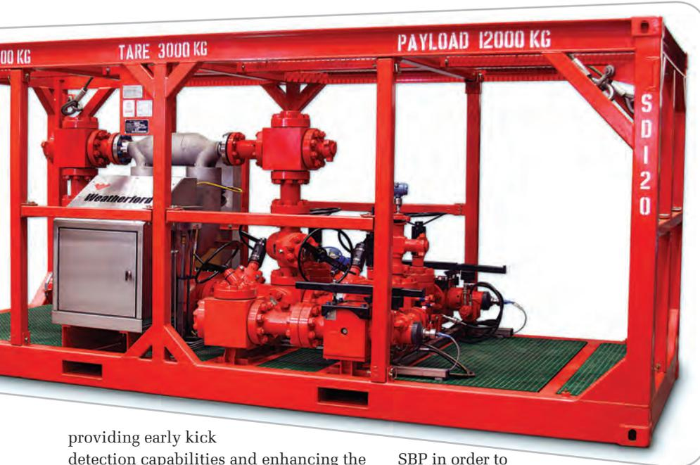
Equipped with a mass flow meter, the MPD manifold is used to achieve precise control of a wellbore's pressure profile while drilling.
