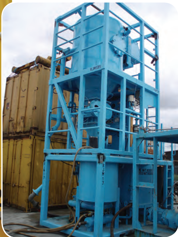
FoundOcean's RJM (recirculating jet mixer).
