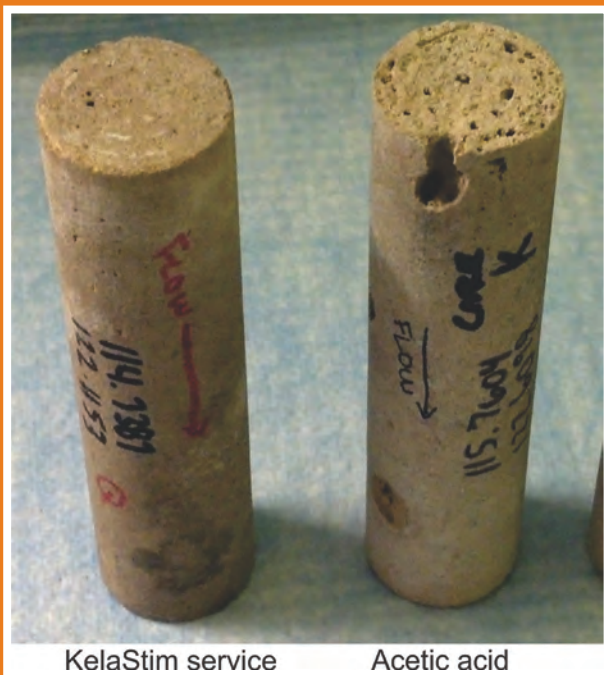
Fig. 3—Example core samples showing treatments with KelaStim service (left) and acetic acid (right) at 350°F. KelaStim service has less risk of formation damage than acid-blend fluids.
