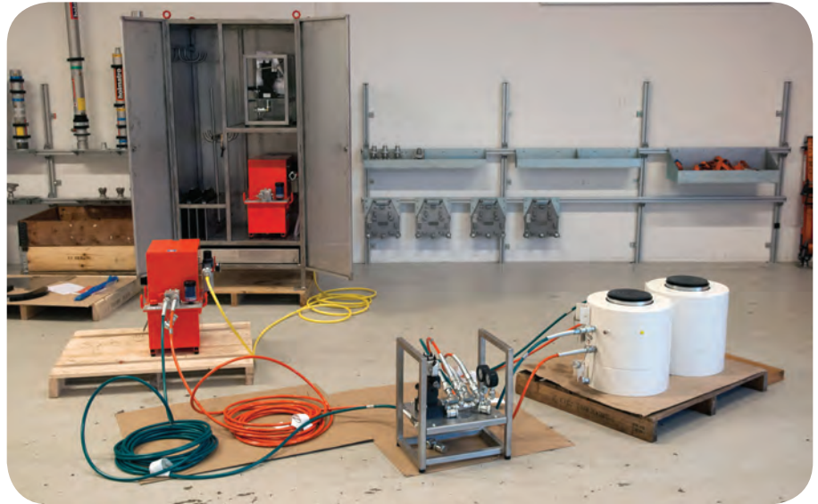
Above: Complete system test set for factory acceptance test. Right: Two 536-tonne capacity hydraulic cylinders, each weighing 400 kilos. Photos from from Holmatro.
