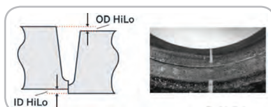
Internal HiLo misalignment between butted pipes.
