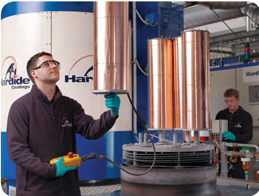
Hardide reactor loading to perform the CVD process. Photos from Hardide Coatings.
