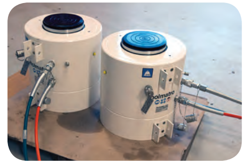
Above: Complete system test set for factory acceptance test. Right: Two 536-tonne capacity hydraulic cylinders, each weighing 400 kilos. Photos from from Holmatro.
