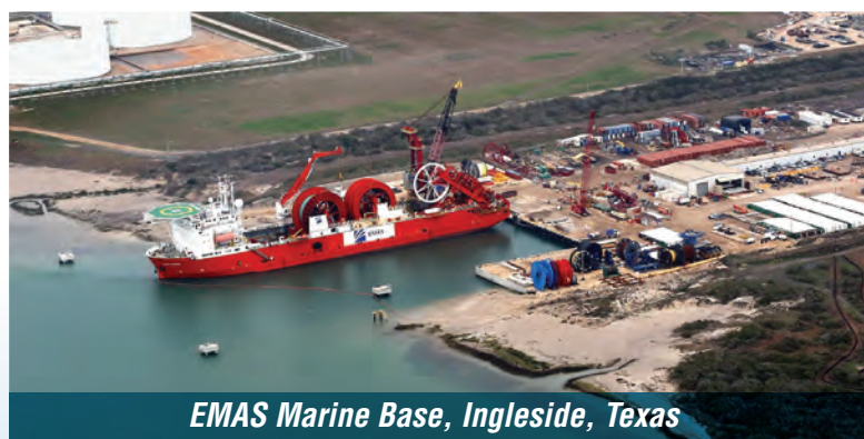
Lewek Constellation - Ultra Deepwater Rigid & Flexible Pipelay/Heavy Lift/Construction Vessel/DP3
