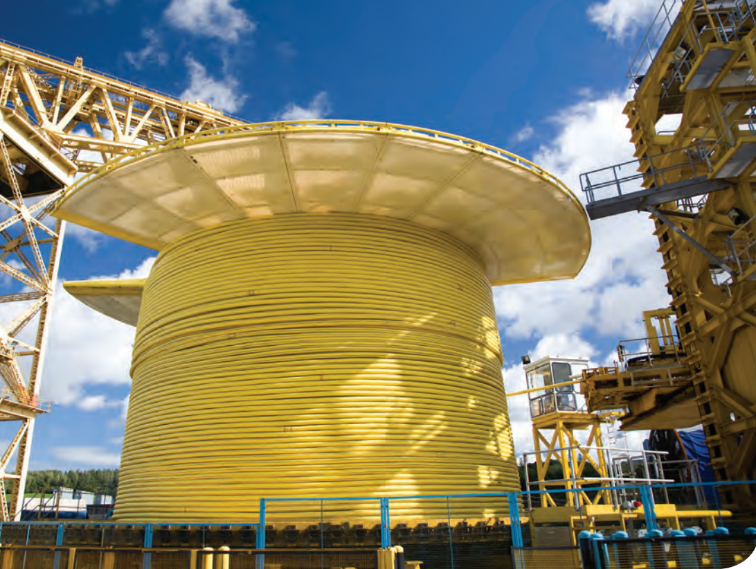
Umbilical spools on Technip Umbilicals' quayside in Newcastle. Photos from Technip.
