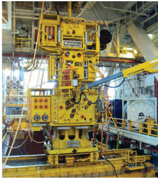
An emergency disconnect and lower riser package. Photo from OneSubsea.
