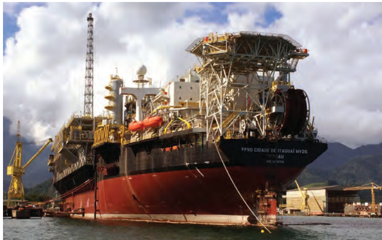
The Cidade de Itaguaí FPSO is the latest vessel to come onstream at Petrobras and BG Group’s Iracema Norte development. Anchored 240km off the coast of Rio de Janeiro, in about 2240m water depth, the FPSO is connected to eight production wells and nine injection wells. Photo from BG Group.
