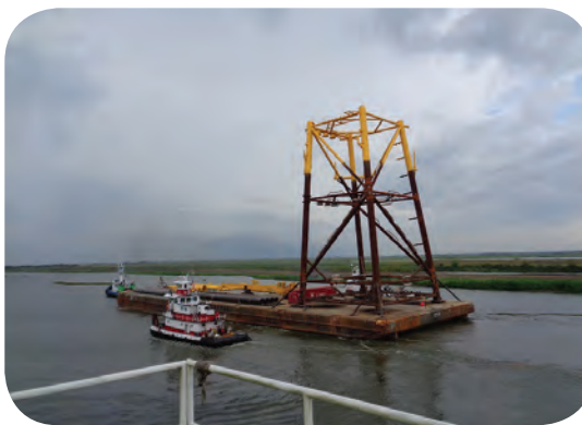
The re-used jacket of the Nenè platform, owned by Eni Congo, during transportation from the US Louisiana yard to offshore Congo. Images from RINA Services.
