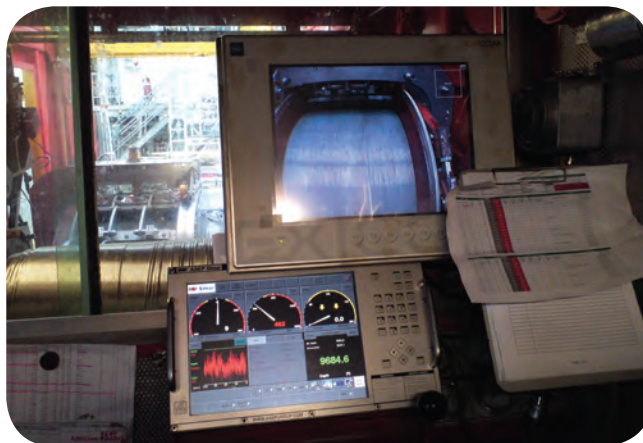
During the operation offshore Norway, the winchman used this panel to monitor the line depth, speed and tension, and the video monitor to verify that the spooling was running properly on the drum. The panel pictured indicates that a line depth of 9684ft has been reached in the well.
