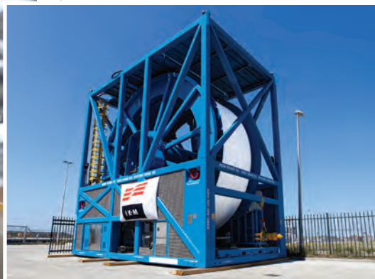
A deepwater downline and reeler package for riserless light well intervention and pipeline pre-commissioning.
