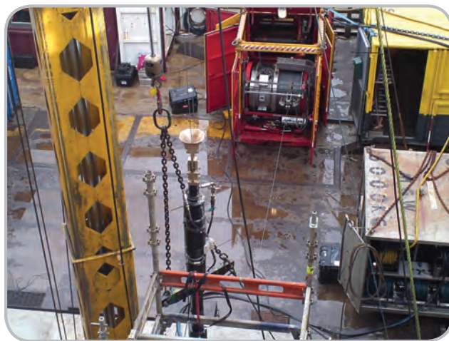
Pictured on the deck is the wireline unit, as it spools the Z-Line out towards the well. It runs under a lower sheave, up and over an upper sheave (not pictured) and down through the brass-colored bend restrictor funnel into the pressure control equipment, and then into the well.
