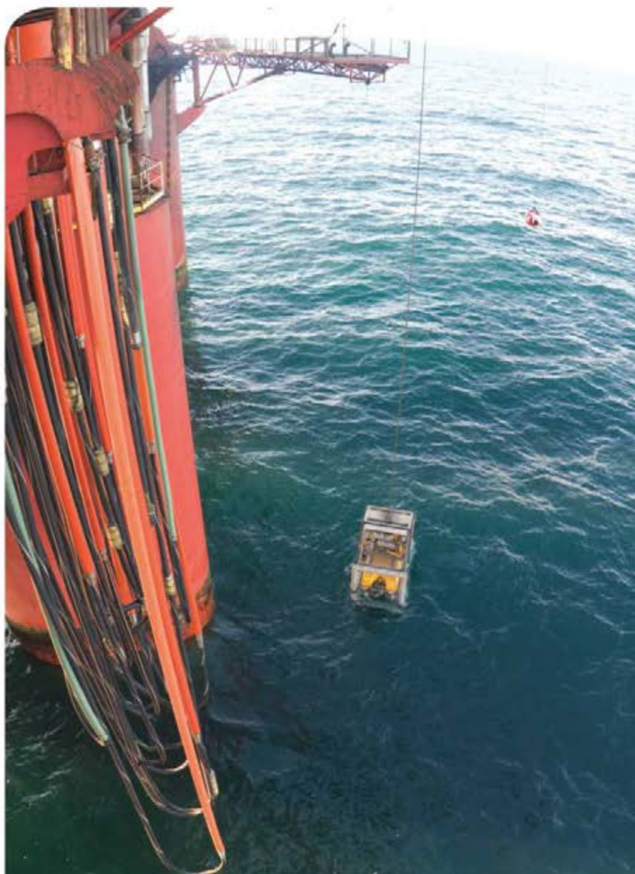
Platform-based ROV being deployed.
