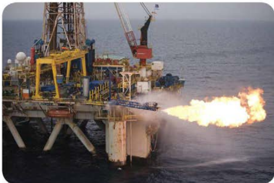
Flare test at the Tamar field offshore Israel. Photo from Delek Group
