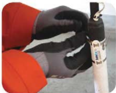
Each equipment is fitted with an RFID chip, approved for Ex zone 1.
