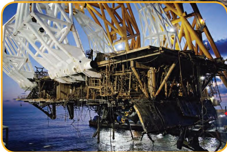
Peter Devine, of Versabar, sent in these photos of the company's heavy lift vessel, *VB 10000*, hard at work. The *VB 10000* decommissions a 2650-ton topside in the Gulf of Mexico. The twin gantries rise 260ft above the waterline. With a rated lift capacity of 7200-tons it is the largest lift vessel ever built in the United States.
