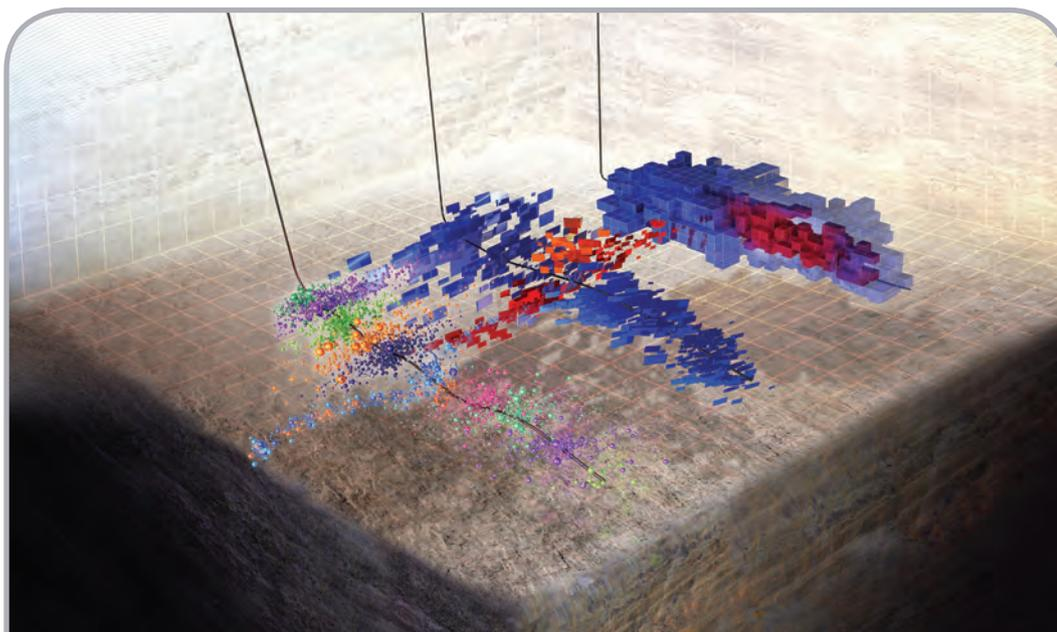
**Microseismic monitoring shows how the reservoir responds to hydraulic fracturing in real time.**
