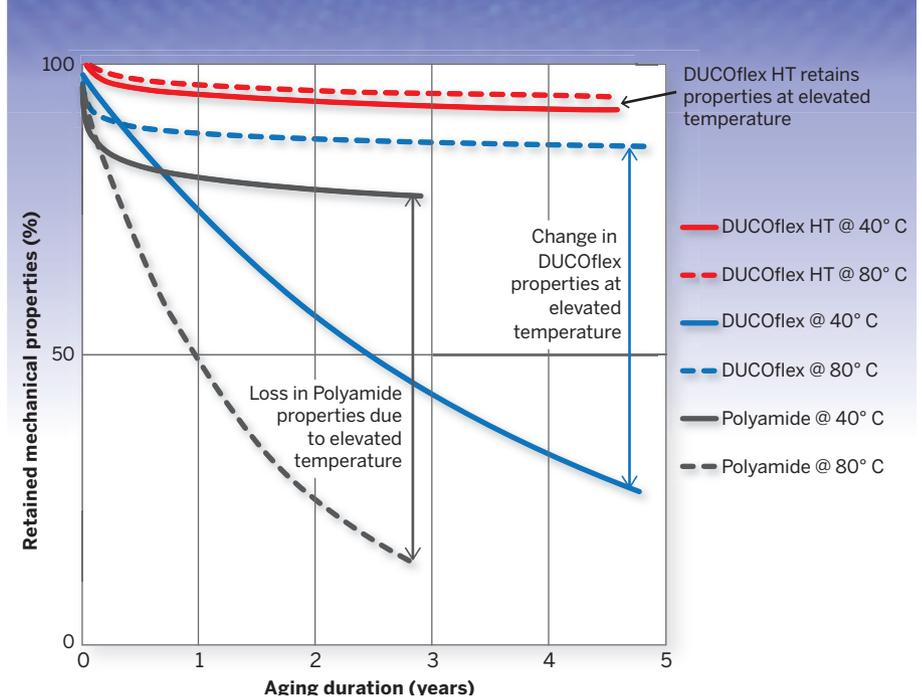
Figure 1 – Traditional hose liner materials vs. DUCOFlex HT.
