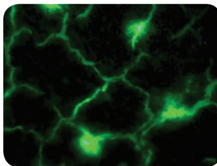
**The smart coating fluoresces in cracks under UV light.**
