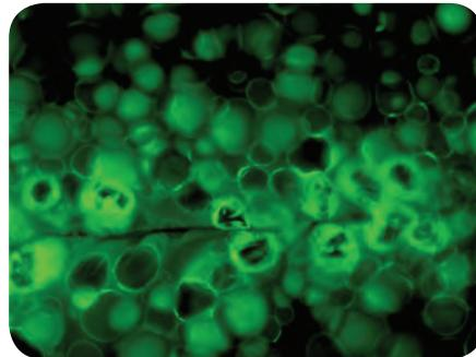
**"Smart beads," filled with chemicals that can fill cracks caused by pipeline corrosion, are added to a coating that is painted on the asset before it is deployed. Terahertz spectroscopy devices enable maintenance personnel to identify where the beads have burst and the pipe requires repairs.** Images from Battelle.
