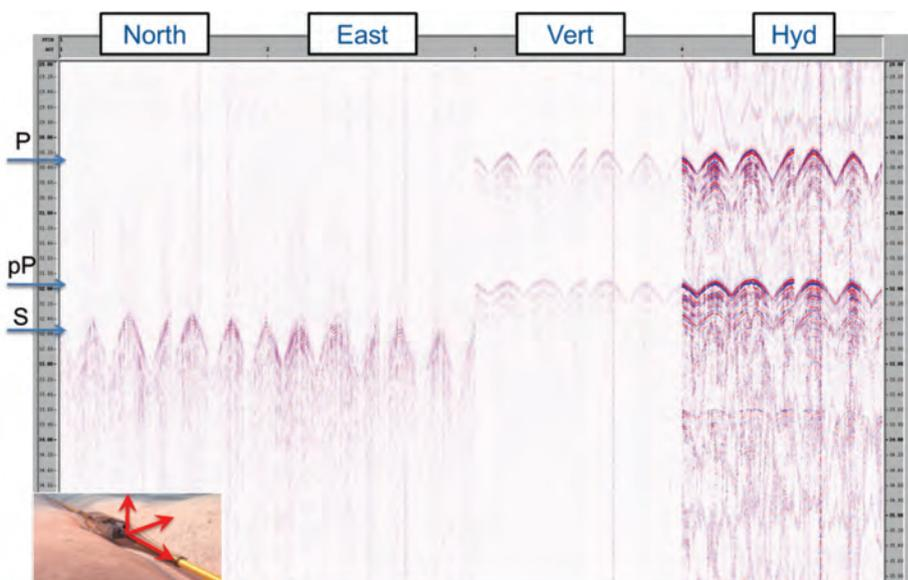
**Fig. 2: Four-component gather of one microseismic event with good signal-to-noise ratio after component rotation. Note the clear separation of P- and S-arrivals between the horizontal and vertical components.**
