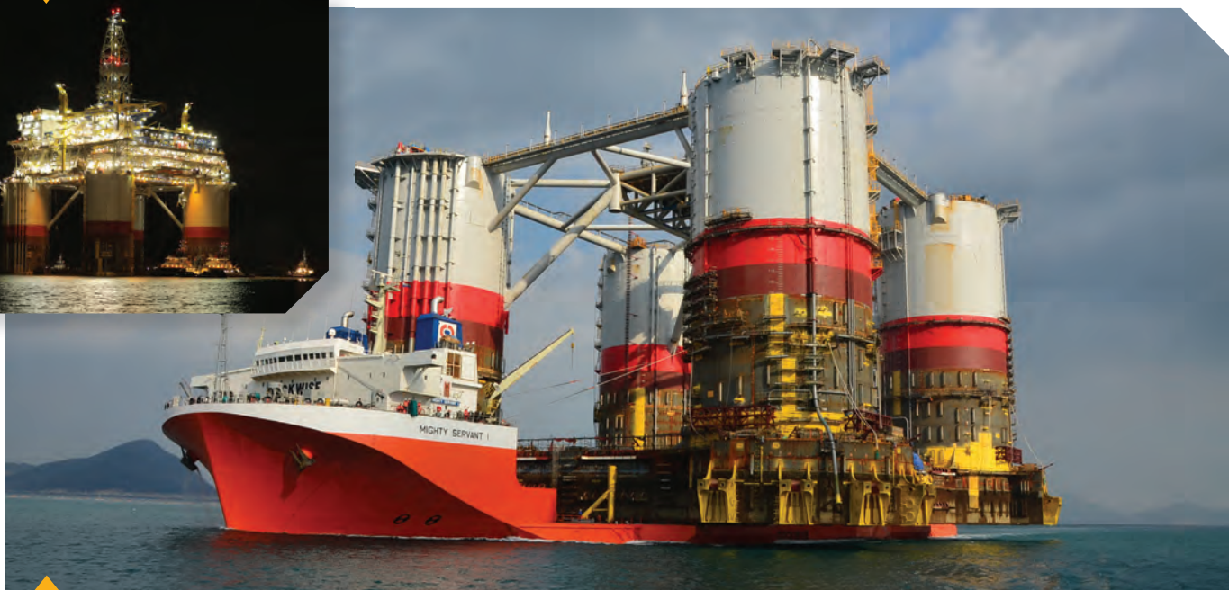
Chevron’s Big Foot platform being towed from Korea to Texas on Dockwise’s Mighty Servant I vessel. Photo from Dockwise.
