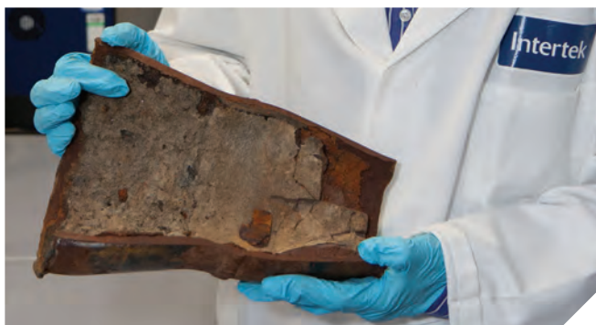
Kevin Harris, Production Chemistry Business Manager at Intertek, examining a pipeline section damaged by scale. Photo from Intertek.
