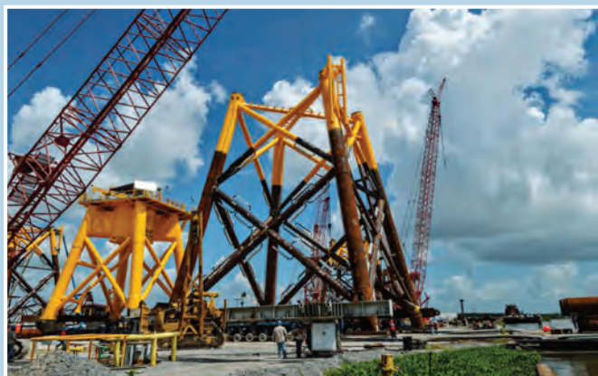
Foundations for Deepwater Wind’s offshore wind farm near Block Island, designed by Keystone Engineering, and built by Gulf Island Fabrication in Houma, Louisiana. This is the US’s first offshore wind farm. Photos from Keystone Engineering.
