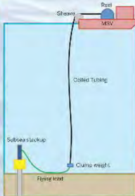
Figure 1 – Traditional vs riserless intervention systems. Images from 2H Offshore.
