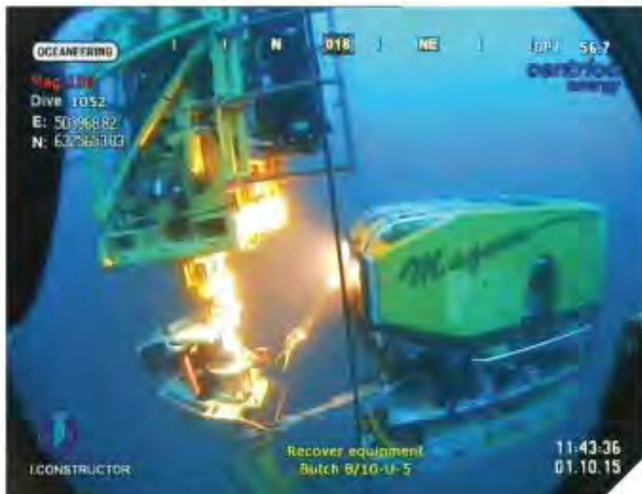
The subsea injector and ROV in operation
